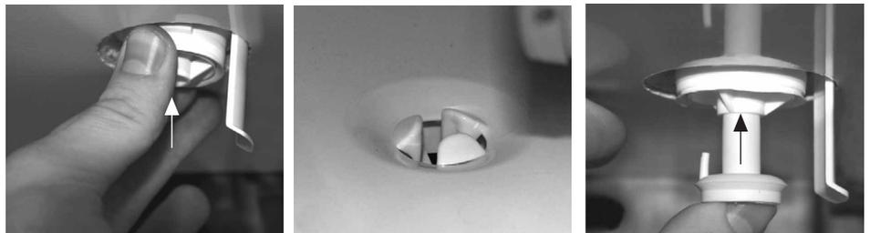
4. Attach siphon casing and engage with a 1/4 turn counter clockwise in the connection element (Ensure that the floater is in the casing!)
