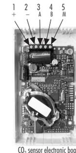
CO<sub>2</sub> sensor electronic board
