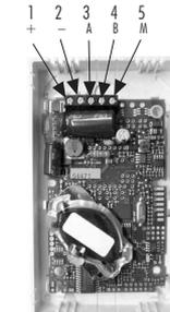
CO<sub>2</sub> sensor electronic board
