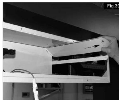
**3.7 Removal of motor unit right**
