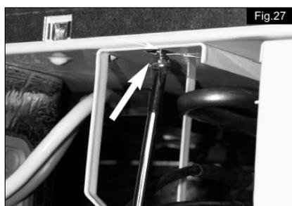
6. Connect electrical connection.
